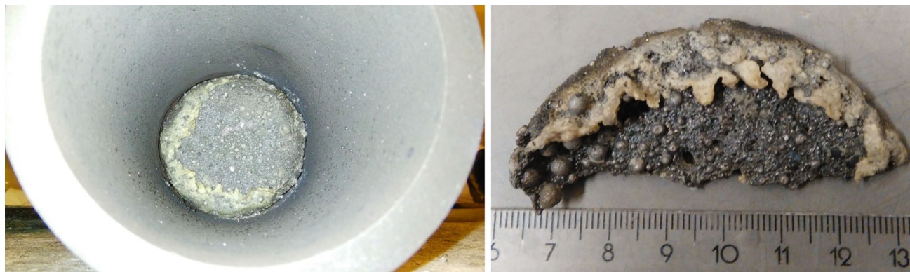
Fig. 8 Representative photographs of the solidified CaC_2 -containing slag: (left) in the bottom of the graphite crucible and (right) removed prior to reaction with water to produce C_2H_2 and PH_3 (color figure online)
