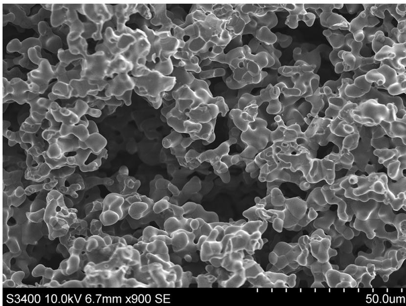
(a) Cross section of porous support
