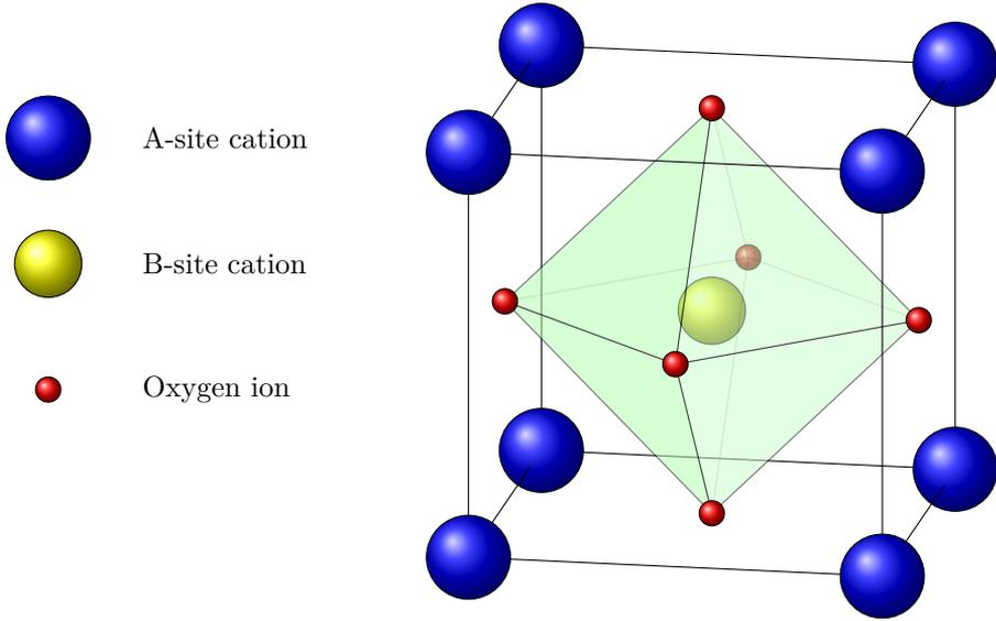
**Figure 2.1:** *Ideal perovskite structure with  $BO_6$ -octahedra and A-site cations placed in interstitial sites*
