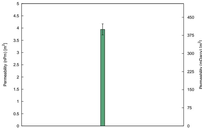
**Figure 4.13:** *Gas permeability of a porous support*
