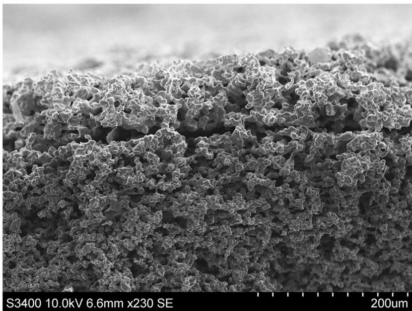
(b) Cross section of porous support
