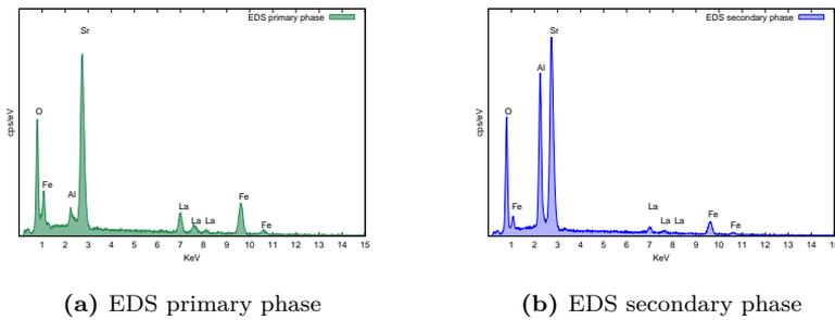
**Figure G.1:** *EDS analysis of the two seen phases from SEM micrograph*
