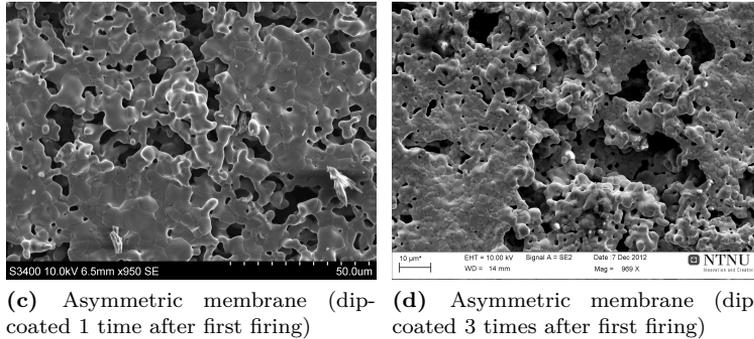
**Figure 5.2:** *SEM micrographs: comparing micrographs of two asymmetric membranes, dip-coated one and three times after the first firing*
