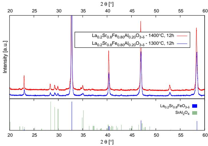
**Figure 4.6:** XRD-pattern of LSFAl2882 made with nano-alumina
