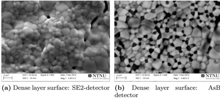
**Figure 5.4:** SEM micrographs: comparing micrographs taken with the secondary electron detector and the backscatter detector
