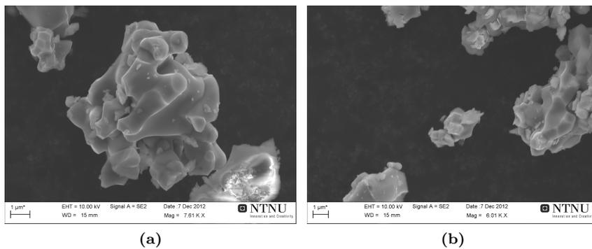
**Figure 4.1:** SEM micrographs of the coarse LSFAl2882 powder. Note the different particle sizes
