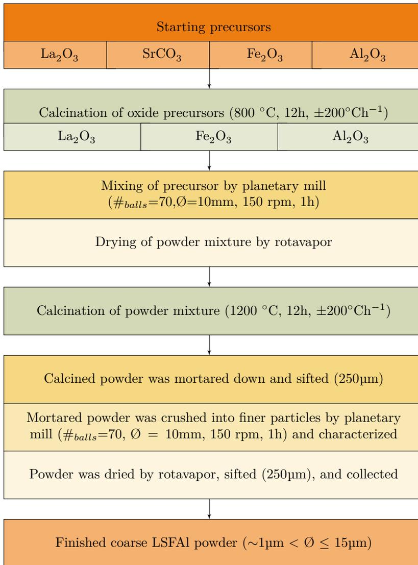
**Figure 3.2:** Flow chart of the LSFAl2882 powder synthesis
