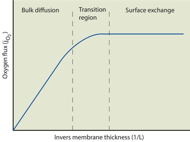
**Figure 2.6:** Illustration of the oxygen flux profile versus membrane thickness
