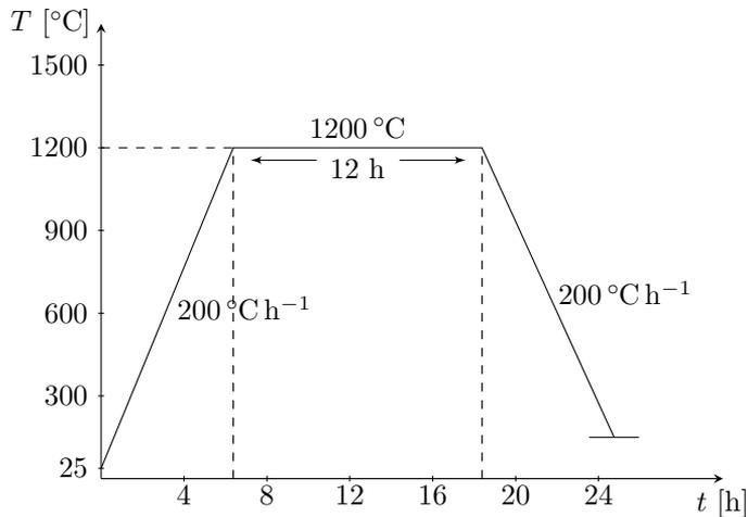
**Figure 3.1:** *Calcination program for solid state synthesis of LSFAl*
