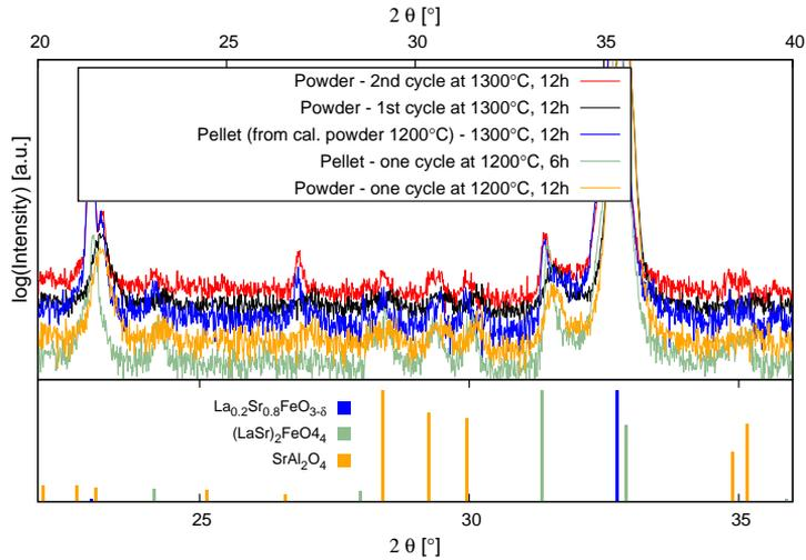
(b) XRD-pattern: Evolution of LSFAl2882 powder with temperature. Note the logscale on the y-axis and the reduced  $2\theta$  area.**Figure 4.4:** XRD-patterns: evolution of LSFAl2882 with temperature
