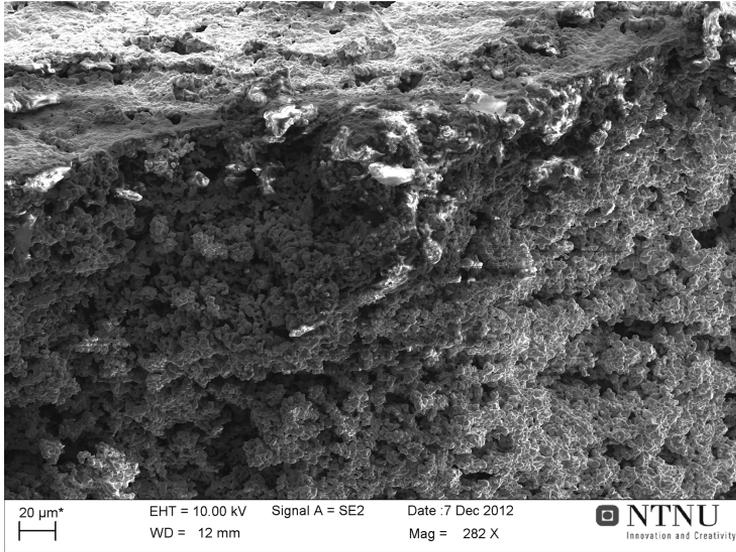
(a) Cross section of the asymmetric membrane
