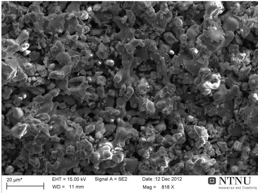
(d) Top surface of the porous support, note the different scale
