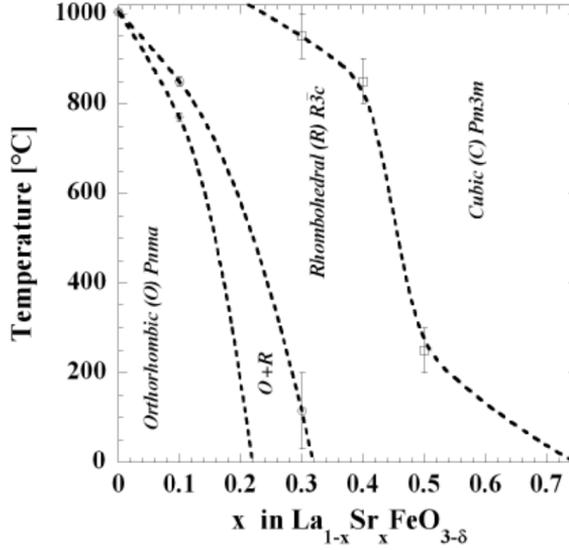
**Figure 2.2:** Pseudo-binary phase diagram of  $\text{La}_{1-x}\text{Sr}_x\text{FeO}_{3-\delta}$ , Figure from [13]
