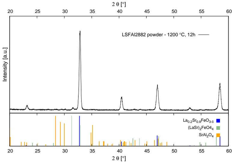
(b) XRD-pattern of coarse LSFAl2882 powder: All undistinctive LSF peaks matched. Note: logarithmic scale on the y-axis
