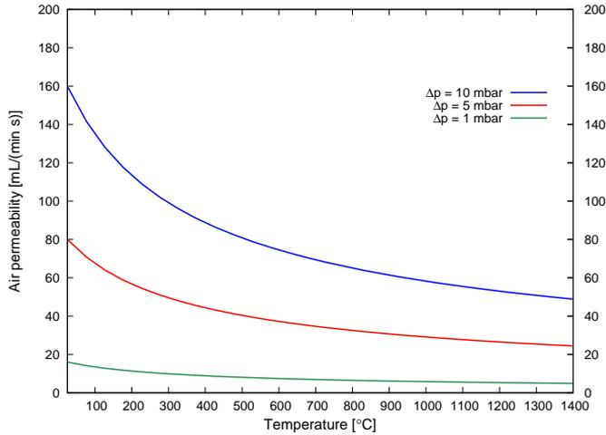
**Figure 4.14:** *Expected gas permeation of the porous support at elevated temperatures for different pressure drops.*
