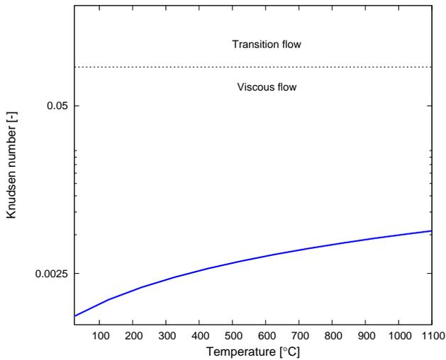
**Figure 4.15:** *Evolution of the Knudsen number with temperature, pressure held constant at  $\bar{p} = 1.005$  bar.*
