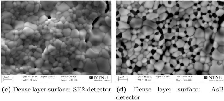
**Figure 4.18:** SEM micrographs: comparing micrographs taken with the secondary electron detector and the backscatter detector
