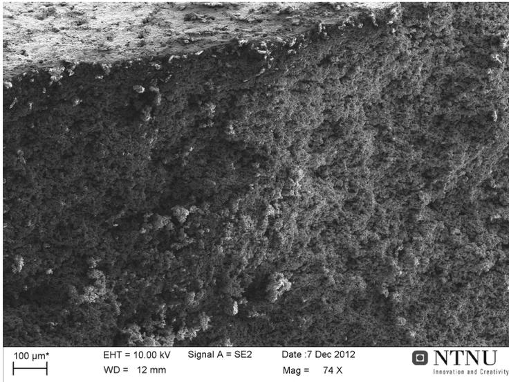
(b) Cross section of the asymmetric membrane
