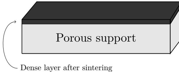
**Figure 3.7:** *Illustration of the dense functional layer ontop of the porous substrate after sintering. Densification has occurred*
