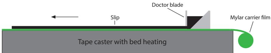
**Figure 3.4:** Illustration of operating principle for a tape caster
