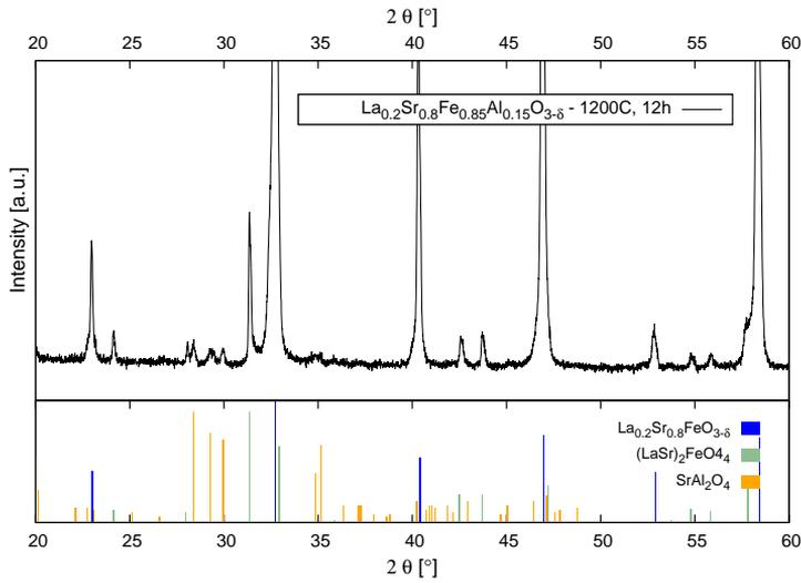
(b) XRD-pattern:  $\text{La}_{0.2}\text{Sr}_{0.8}\text{Fe}_{0.85}\text{Al}_{0.15}\text{O}_{3-\delta}$ **Figure 4.5:** XRD-patterns: Different compositions of LSFAL, note the different compositions in a) and b).
