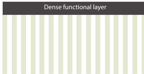
**Figure 2.7:** *Illustration of an asymmetric membrane showing the dense functional layer ontop of a porous support (Note: not in scale)*
