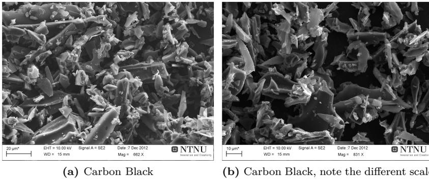
**Figure 4.2:** SEM micrographs of the carbon black powder used as a pore former after 30 minutes of ball milling. Note the many different shapes and sizes.
