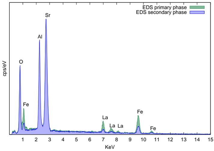
**Figure G.2:** *EDS analysis of the dense layer of the asymmetric membrane*
