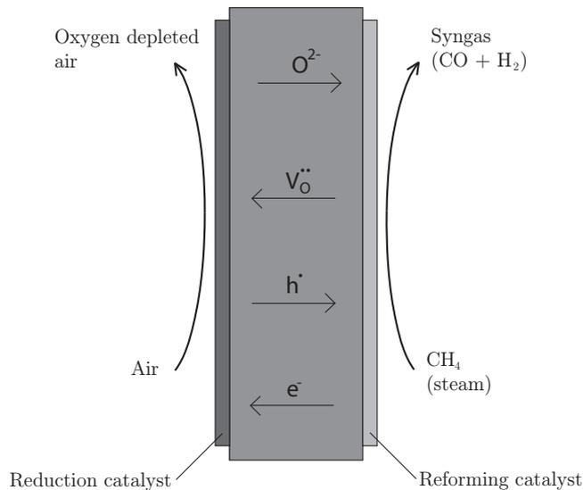
**Figure 2.5:** Illustration of oxygen transport through a MIEC-membrane in the partial oxidation of methane to produce syngas, Figure redrawn from [1].
