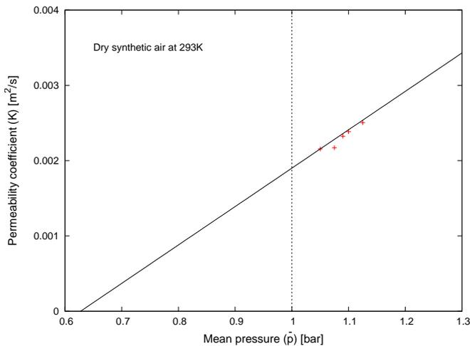
**Figure 4.12:** *Permeability coefficient of a porous support*
