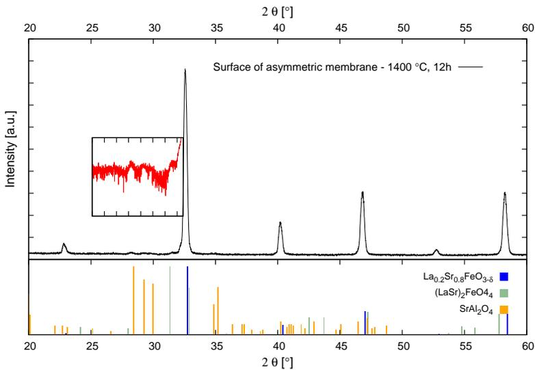
**Figure 4.16:** XRD-pattern of the sintered asymmetric membrane. The XRD measurement was done on the surface of the dense functional layer. Note the highlighted region (in red) exposing the presence of  $\text{SrAl}_2\text{O}_4$ .
