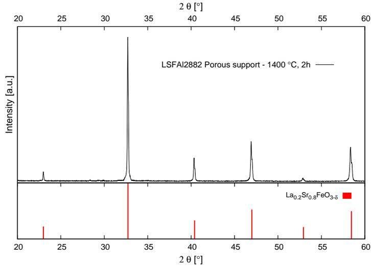
**Figure 4.9:** XRD-pattern of the sintered LSFAl porous support (support was crushed for XRD measurement)
