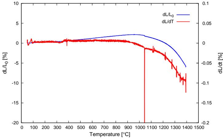
Figure 4.7: Dilatometry curve for LSFAl2882
