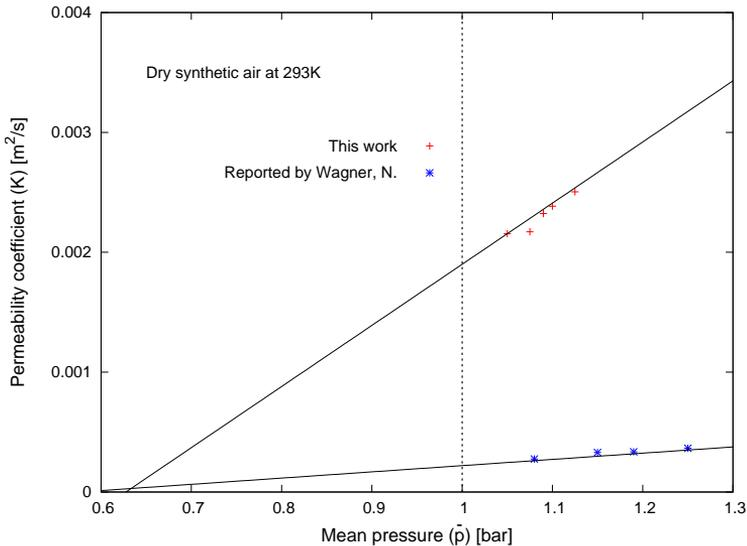
**Figure 5.1:** Comparison of the gas permeability of a porous support produced by tape casting (this work) and by uniaxial pressing (Wagner, N. [7])
