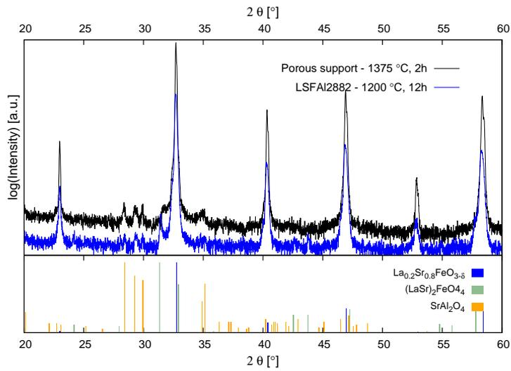
**Figure 4.10:** XRD diagram of the calcined LSFAl powder and powder from the porous support (crushed after firing). Note the logarithmic y-axis
