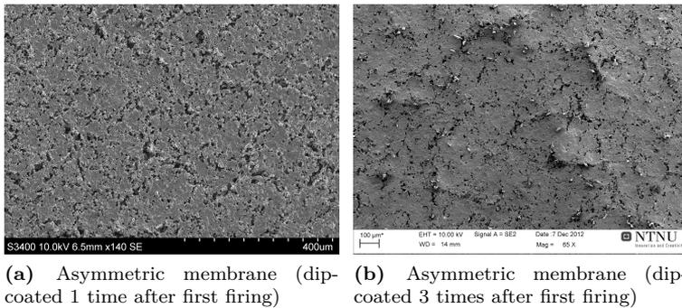
**Figure 4.19:** SEM micrographs: comparing micrographs of two asymmetric membranes
