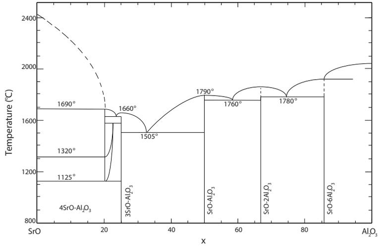
**Figure 2.4:** Phase diagram of the  $SrO-Al_2O_3$ -system, Figure redrawn from [19]
