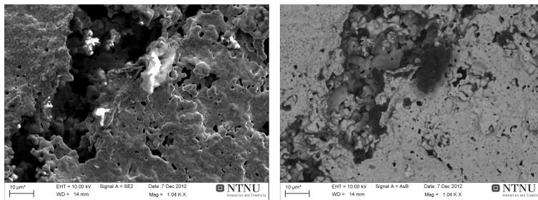
(a) Dense layer surface: SE2-detector (b) Dense layer surface: AsB-detector
