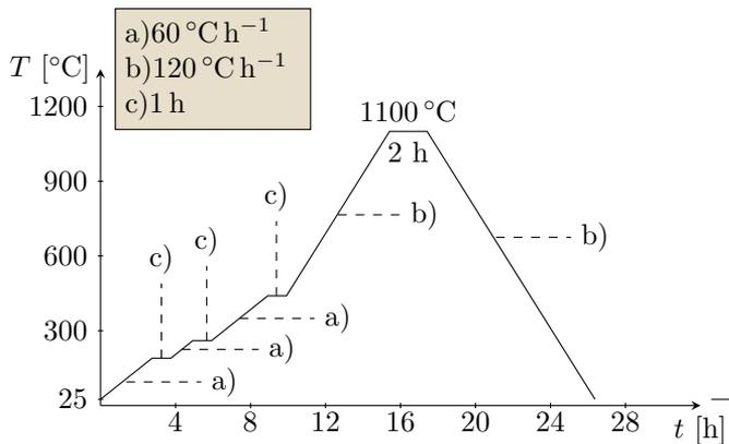
**Figure 3.5:** Calcination program for the porous support, dip-coated once.
