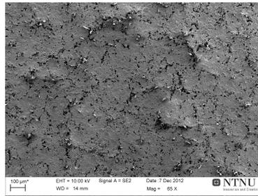
(b) Asymmetric membrane (dip-coated 3 times after first firing)
