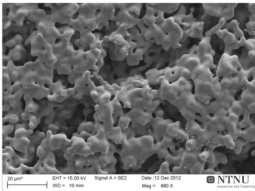
(f) Bottom surface of the porous support, note the different scale
