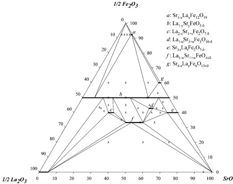
**Figure 2.3:** Isothermal phase diagram of the ternary system  $\text{La}_2\text{O}_3\text{--SrO--Fe}_2\text{O}_3$ , from [17]
