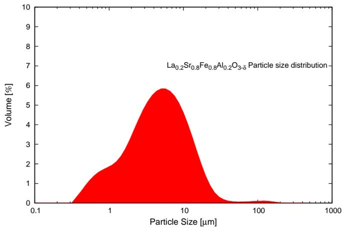
Figure 4.8: Particle size distribution of coarse LSFAl produced by the solid-state reaction
