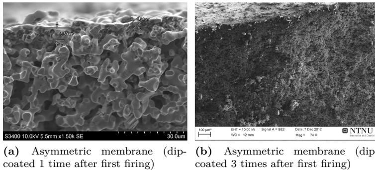
**Figure 5.3:** *SEM micrographs: comparing micrographs of two asymmetric membranes*
