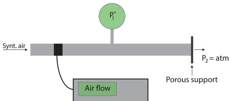
**Figure 3.8:** *Illustration of experimental setup for air permeation measurements of the porous supports*
