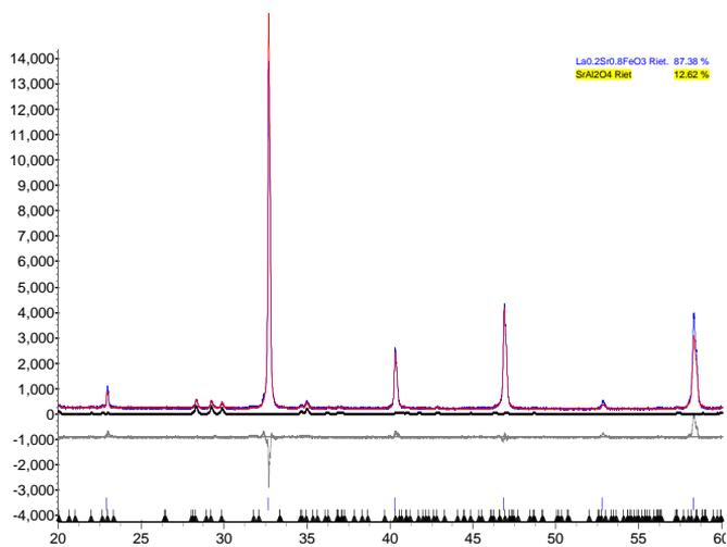
(f) Topas analysis of the LSFAL powder prepared with nano-alumina (matched with cubic LSF)
