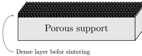
**Figure 3.6:** *Illustration of the thin functional layer ontop of the porous substrate after dip-coating.*
