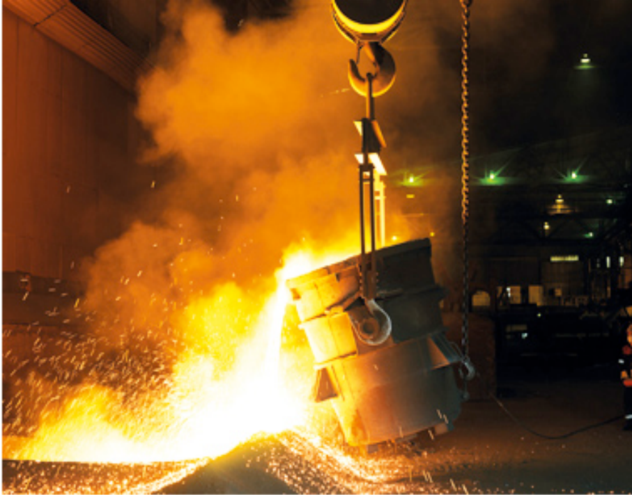
Figure.A.4. Liquid silicon metal flows out of ladles onto a bed of silicon sand, where it can cool and solidify [21].
