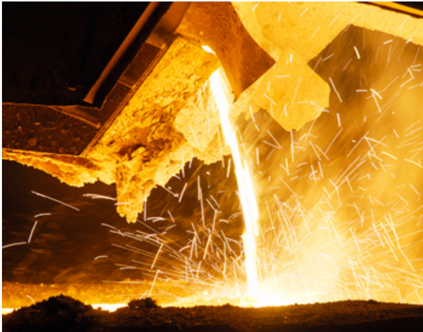
Figure. A.5. Liquid silicon, which after cooling will be taken to the crusher [21].
