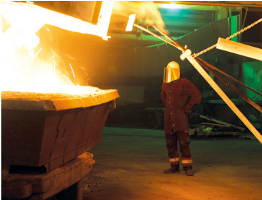
Figure.A.3. The carbon in the coal removes the two oxygen atoms from the quartz-leaving liquid metallurgical-grade silicon [21].
