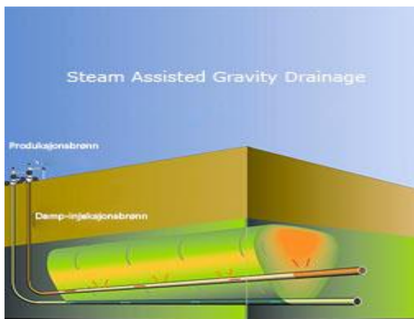
Figur 2.4. Prinsippet for SAGD
