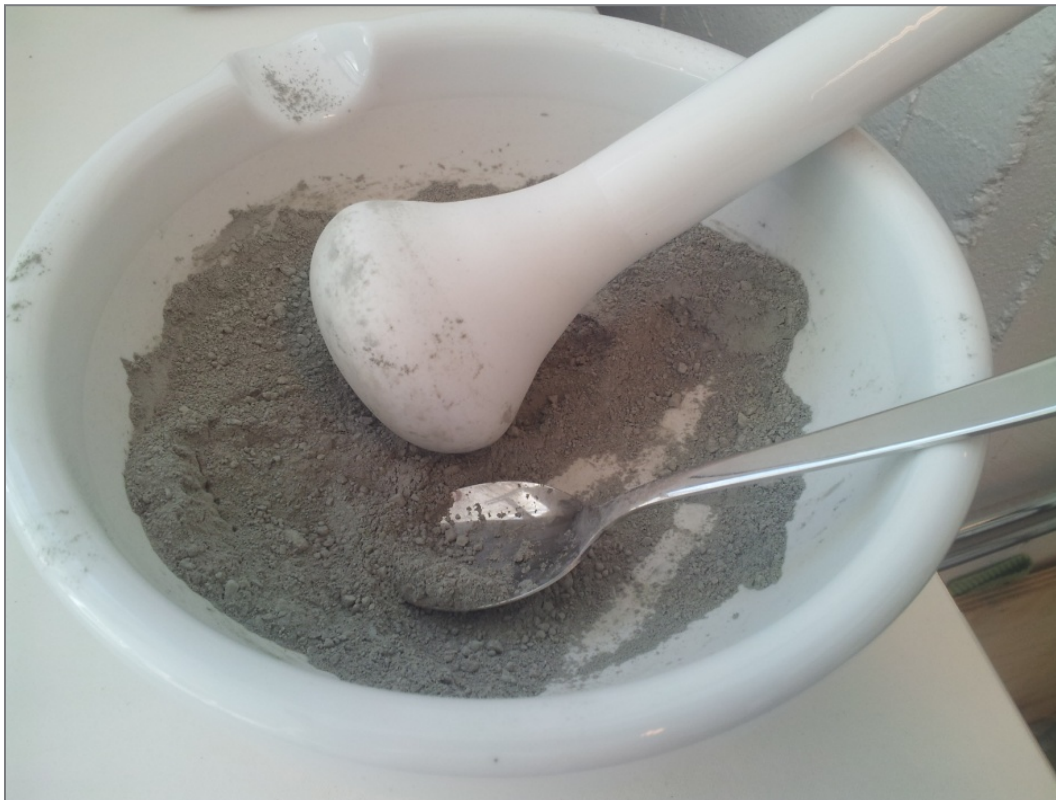
Figure 3.3 - Grinding of dried clay from Buvika to make a fine powder for use in the experiments (Lisbet Sørensen, 22.02.2012)
