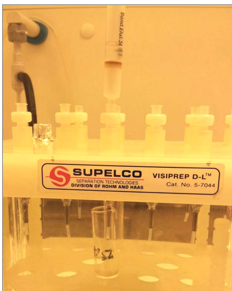
Figure 3.8 - Bond-Elut clean-up of sediment extracts on a 500 mg Si-column, n -hexane used as solvent and eluent (Lisbet Sørensen, 30.09.2011).
