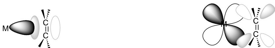
Figure 2.3 a) Vacant d orbital, filled \pi on ligand acting as \sigma -donor b) Filled d orbital, empty olefin \pi^* orbitals
