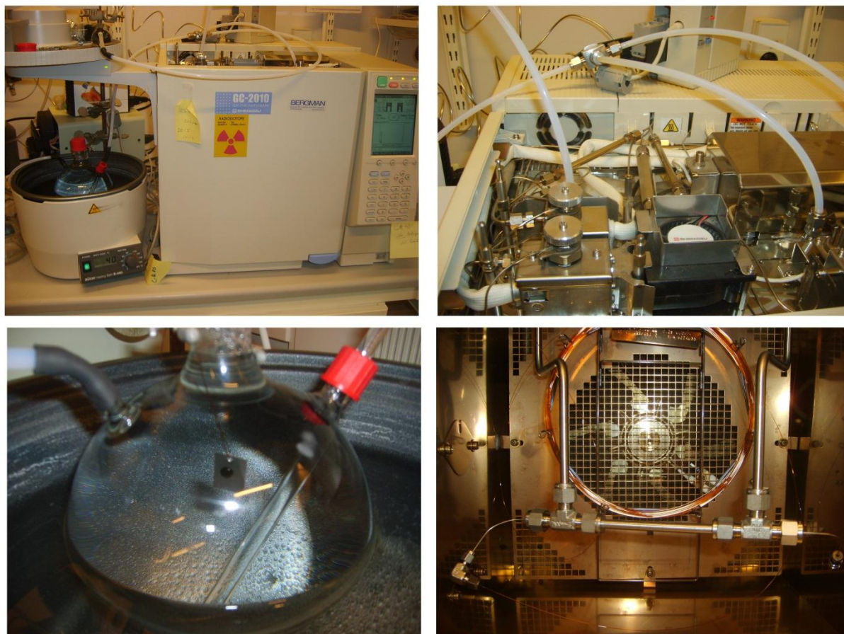
Figure 3.2: Overview of the MIFID system for water analysis. A) An overview of the whole setup. A flask with water is placed in a water bath and connected to the MI in a GC oven by Teflon tubing. B) The top of the GC: The tube to the right introduces the sample to the membrane, and the tube to the left returns the samples to the flask. The tubing to the far right is used to introduce clean air/water via the 3-way Ball valve in the back. C) Oil sample spread on a piece of aluminum foil in the flask. D) Inside view of the GC oven: The sample flow is introduced from right to left, in the horizontal metal tubing, while the hydrogen gas in the membrane tubing inside the interface flows from left to right.
