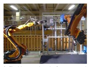
Fig. 3: The lab setup where the floor mounter robot is equipped with a stereoscopic camera.
