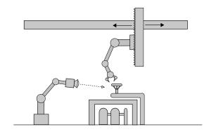
Fig. 1: An illustration of the robot monitoring system. The leader robot is performing a task while the follower robot is monitoring the operation.
