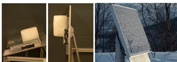
Fig.18. Snow/ice slab firmly sticking to the glass surface of an insulated window pane even at an inclination angle of 90° during a laboratory experiment (left). Snow covering a solar cell panel at an inclination angle of 70° (right) [69,70].
