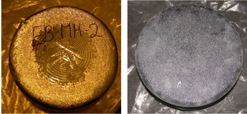
Figure 30: The surface of MH2 (left) and the bottom of MH1 (right) in as-cast ingots
