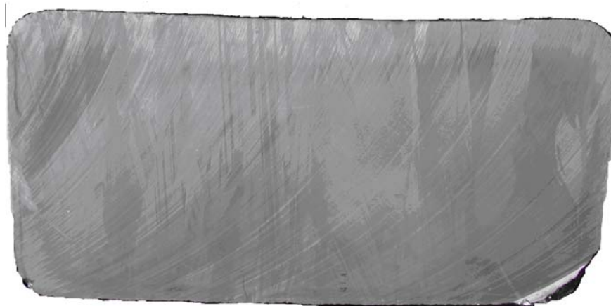
Figure 31: A cross-section picture of ingot MH2. The curved lines are from the cutting.
