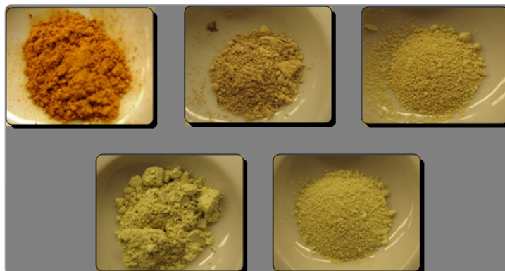
Figure 6.2: A picture of the V_2O_5 /ZSM-5 and V_2O_5 /Y and bulk V_2O_5 . The bulk V_2O_5 is shown to the left at the top. The as prepared V_2O_5 /ZSM-5 is shown on the top to the left. The calcined V_2O_5 /ZSM-5 is shown to the right from the top. The as prepared and calcined V_2O_5 /Y is shown at the bottom left and right respectively.
