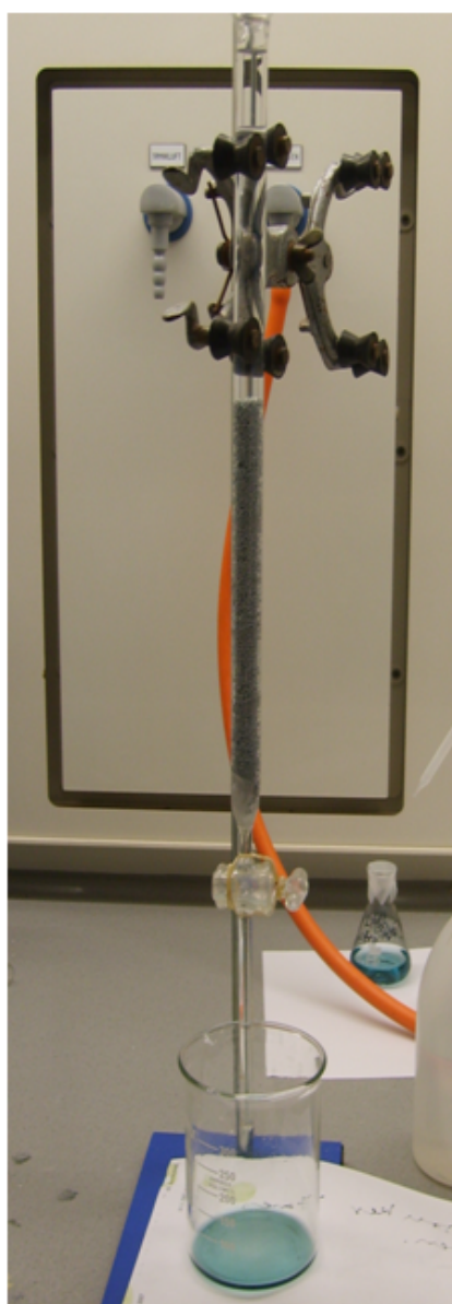
Figure 2.1: The Jones reductor used for the reduction of vanadium.
