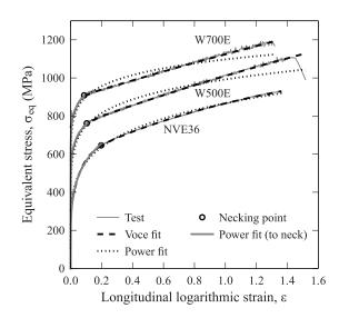
Figure 6. Bridgman corrected stress for NVE36, Weldox 500E, and Weldox 700E.
