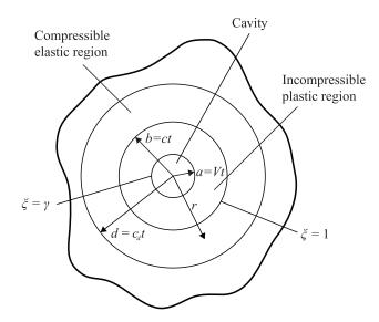
Figure 2. Cavity expansion approximation and different response regions.
