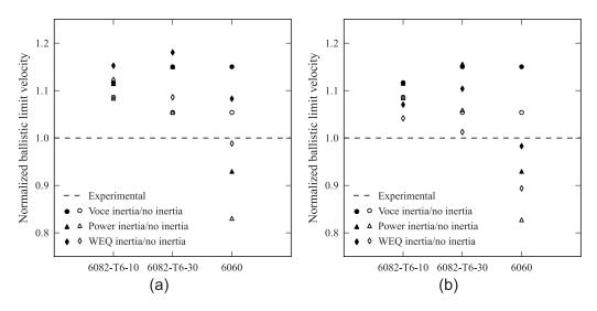
**Figure 8.** Results from CCET analyses on the AA6082 and AIMgSi aluminum alloys: (a) shows results for calibration up to fracture and (b) shows results for calibration up to neck.
