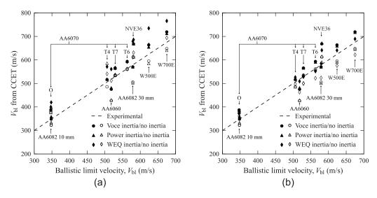
**Figure 10.** Results from CCET analyses for all investigated materials: (a) shows results for calibration up to fracture and (b) shows results for calibration up to neck.
