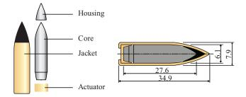
Figure 1. Schematic drawings and geometry of the 7.62 mm bullet (dimensions in mm).
