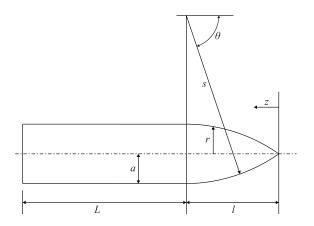
Figure 3. Ogival nose projectile with geometry.
