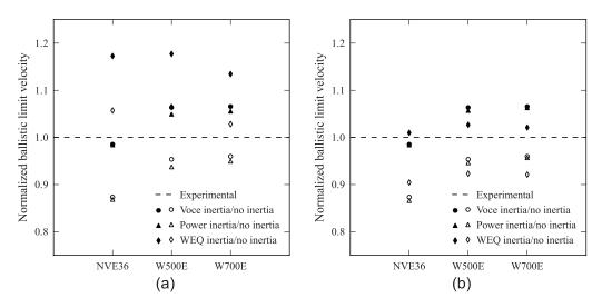
Figure 9. Results from CCET analyses on the NVE36, Weldox 500E, and Weldox 700E steel alloys: (a) shows results for calibration up to fracture and (b) shows results for calibration up to neck.
