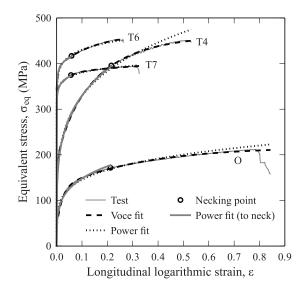
Figure 4. Bridgman corrected stress for AA6070 tempers.
