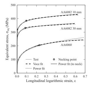
Figure 5. Bridgman corrected stress for AA6060 and AA6082-T6.
