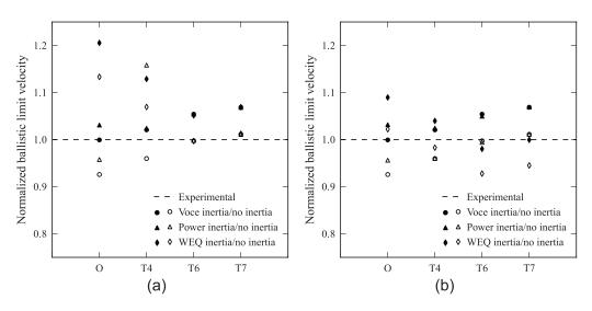
Figure 7. Results from CCET analyses on the AA6070 aluminum alloy: (a) shows results for calibration up to fracture and (b) shows results for calibration up to neck.
