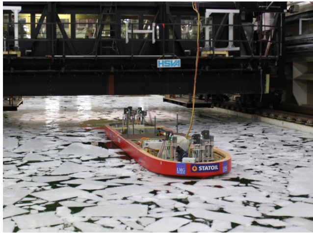
FIGURE 7. The model scale Arctic Drillship during experimental testing at HSWA. Courtesy of DYPIC.
