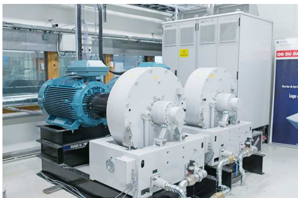
FIGURE 9. Electric motors and eddy current brakes of the HML at NTNU.
