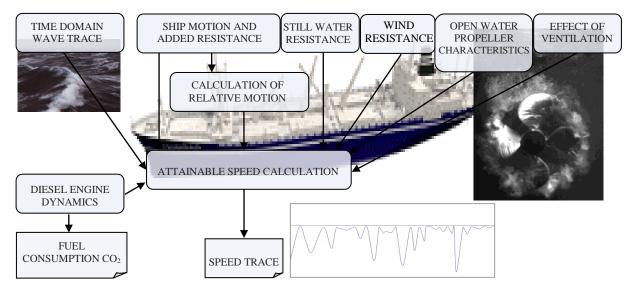
Figure 1. Scheme of the computations of ship speed in a given sea state
