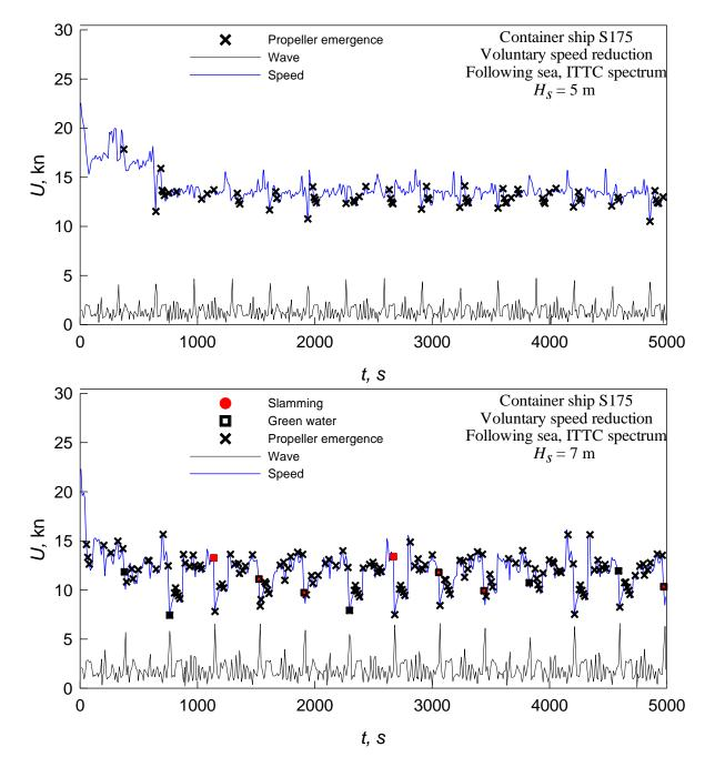
Figure 3. Time trace of ship speed in following sea
