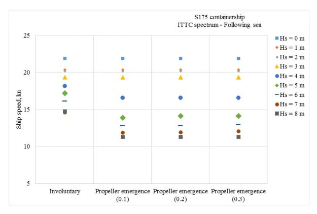
Figure 15. The effect of propeller emergence limiting value on attainable ship speed (following sea)
