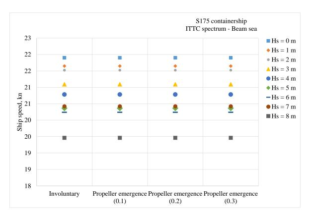
Figure 21. The effect of propeller emergence limiting value on attainable ship speed (beam sea)
