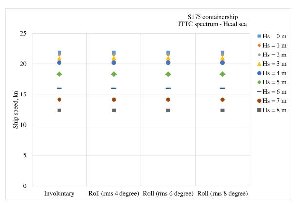
Figure 10. The effect of roll limiting value on attainable ship speed (head sea)
