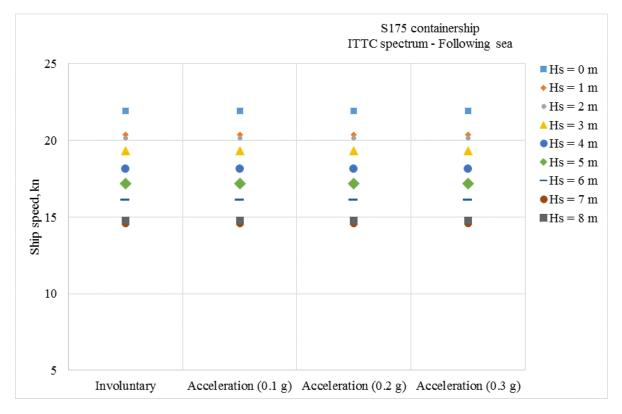
Figure 14. The effect of acceleration limiting value on attainable ship speed (following sea)
