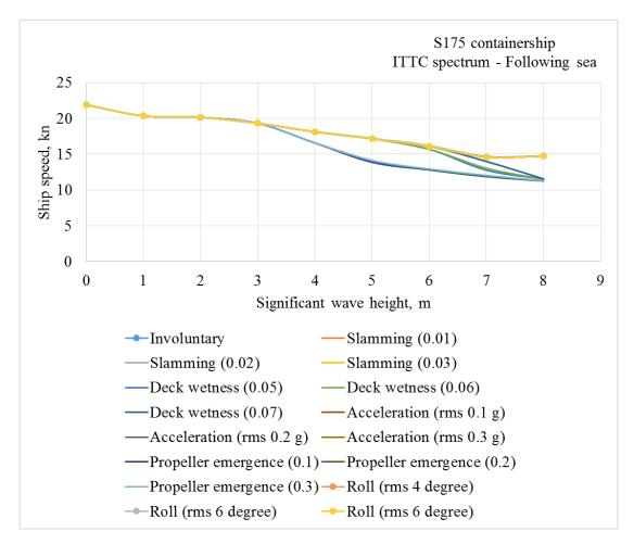
Figure 11. Ship speed loss for following sea
