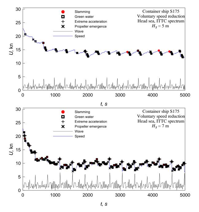
Figure 2. Time trace of ship speed in head sea
