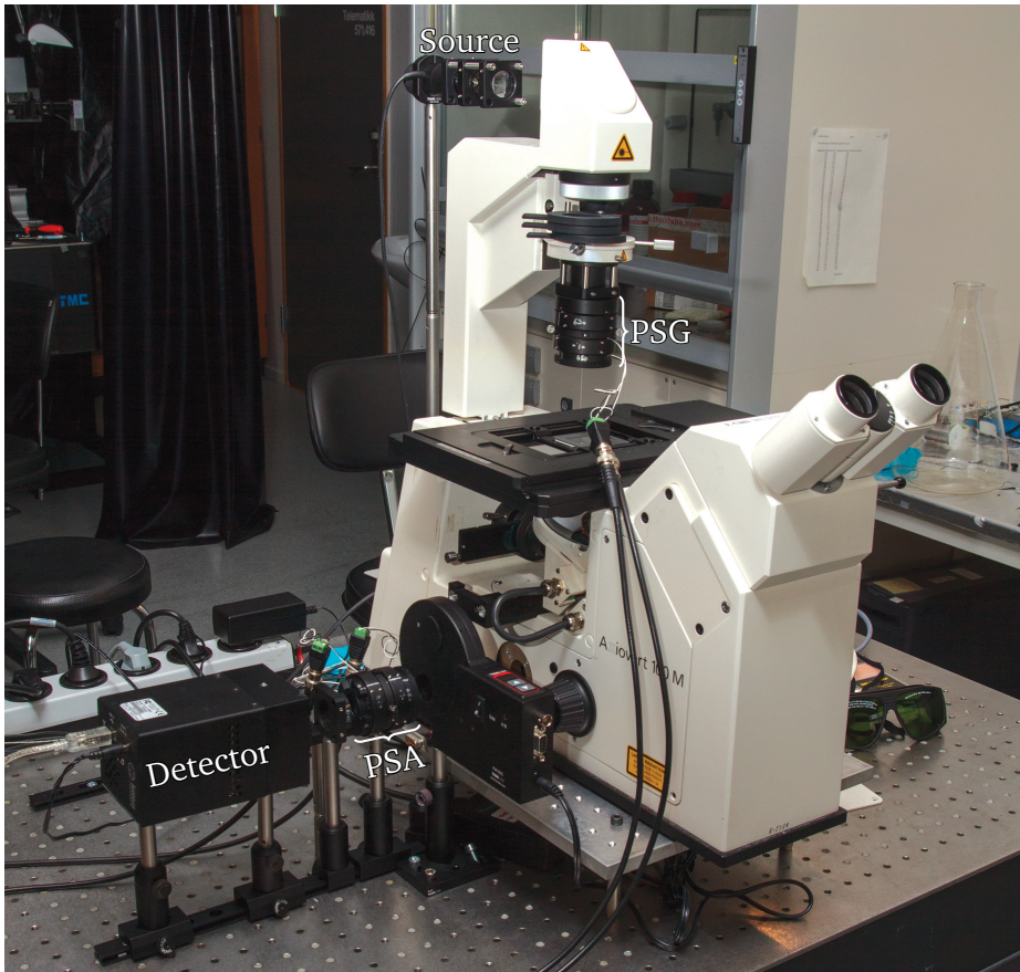
Figure 7.9: Photograph of the prototype Mueller matrix imaging microscope with some parts indicated.
