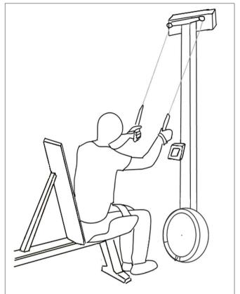
**FIGURE 1** | Test set-up with the participant in a sitting position, strapped around the hips and thighs, in front of the Concept2 ski-ergometer.
