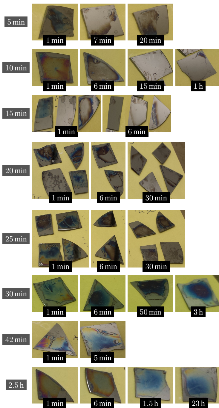
Figure 4.27: Solubility test of unbaked high-PVA stabilized in sodium sulfate for various lengths of time. Color fill legend: black: water exposure time, grey: sulfate exposure time.
