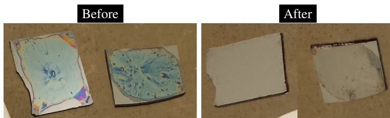
Figure 4.33: Demonstration of water solubility of PAA-films. PAA concentration: 5%. Water exposure time: 1 min. Images are from before and after water exposure. Within each subfigure – left: unbaked sample, right: baked sample.
