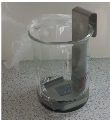
Figure 3.5: Wafer sample kept in solution with custom made device for quick and easy lowering
