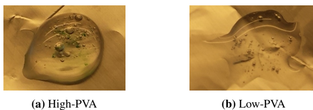
Figure 4.24: Saturated borate induced hydrogels made from both high-PVA and low-PVA. Borate: pH = 10.
