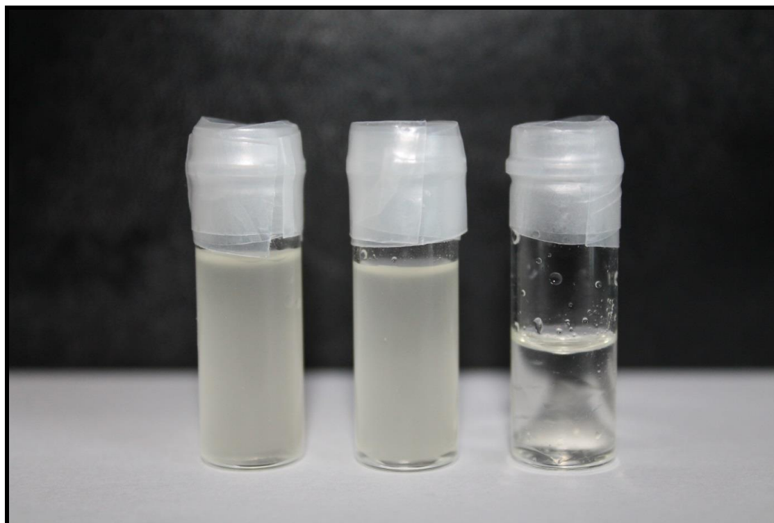
Figure 4.15: Sampled collected in the small glass ampoules. From left to right, emulsion with 2%, 1.5% and 0.5% Laponite RD concentration at constant 0.1 M salt. The stable emulsions found with higher clay concentrations. The appearances of the emulsions are after one week of preparation.
