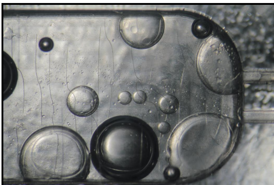
Figure 4.8: Very unstable droplets in the reservoir when the viscosity of the continuous phase (silicone oil) is 100cSt. Dispersed phase is 2% Laponite RD and 0.1 M NaCl in water.
