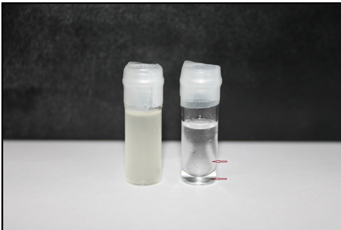
Figure 4.10: Sampled collected in the small glass ampules. Left, stable water in oil emulsions by using castor oil as continuous phase. Right, unstable water in oil emulsions by using silicon oil as continuous phase. In both cases Laponite concentration is 2% and salt concentration is 10^{-1} M. In unstable water in oil emulsions by using silicon oil as continuous phase, we found two clear, separate water (down) and oil (up) phase which are marked by arrow (red) signs. The appearances of the emulsions are after one week of preparation.
