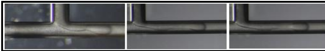
Figure 4.6: (a) Microphotograph of formation of plugs at low value of Ca ( 4.7 \times 10^{-3} ). The sharp breakup of droplet plugs due to the domination of the interfacial tension at low flow rates u (21mm) (b) microphotograp of flow that is in transition to laminar flow. By increasing the flow rates (41mm) and the Ca number ( 8.9 \times 10^{-3} ), the disperse phase flow a bit into the horizontal channel and forms a neck before the plugs are sheared off. (c) Microphotography of flow where long neck is formed and plugs sizes become smaller when the flow rates (58mm) and Ca ( 1.2 \times 10^{-2} ), increases further. This is due to the relative viscous force becomes more dominant and the interfacial tension force is not sufficient for sharp plugs breakups. For all picture, Q_c is silicon oil (10cS) and Q_d , De-ionized water with 1m%clay. length of the laminar segment is 2mm.
