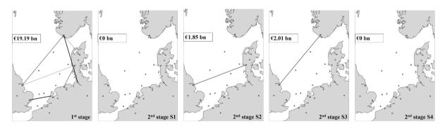
Fig. 5. Multi-stage stochastic program solutions. The first stage investments in the most-left figure, followed by second stage investments ranging from scenario 1-4. The system planner has the option to postpone investments, typically the ones that only occur in particular scenarios. Investment costs are given in the figure.
