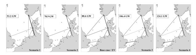
Fig. 3. The plots shows the different solutions obtained from a deterministic program for four different wind capacity scenarios, in addition to the expected value (EV) scenario, i.e. the base case. The thickness of the line plots indicate the size of the investments. Offshore wind capacity and scenario number are labeled in each plot.
