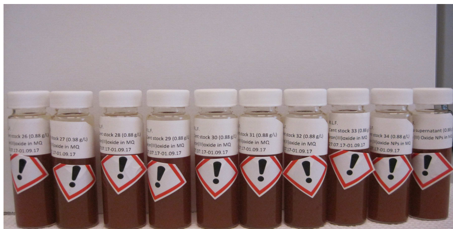
Figure 6.9: Turbidity of the supernatant for the mass produced \text{Fe}_2\text{O}_3/\text{PEI} MNP
