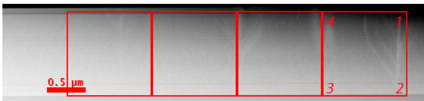
Figure 4.11: A schematic of the attempt to measure the defect density in each sample. The numbers indicate the 4 positions where the thickness was measured, and the red squares is the area being imaged.
