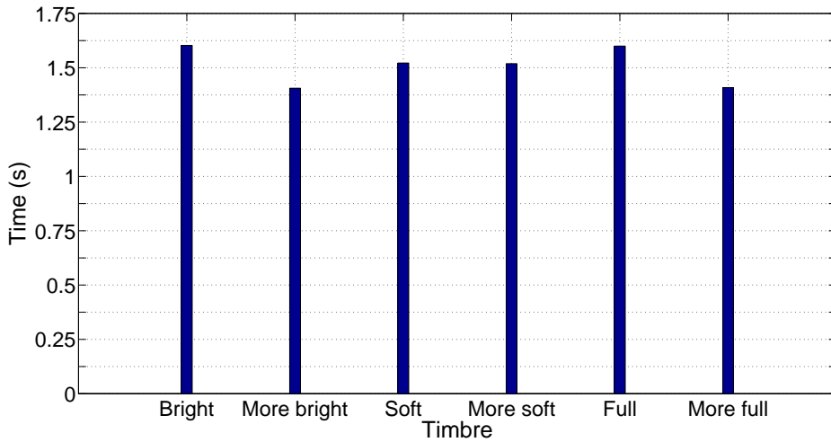
Figure 3.14: Inter-onset interval for the first and second onset of measure 24. Estimated uncertainty is \pm 5 ms.
