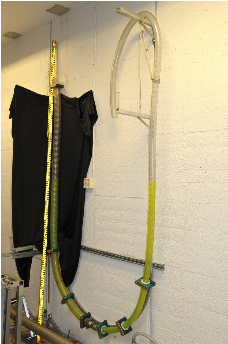
Figure 3.3: The experimental setup for the U-tube with an inner diameter change. The tubes are joined at the bottom; the diameter of the left leg is 6cm while the diameter of the right leg is 4cm. The reinforcing steel wire in the tubes can be seen as the horizontal lines in each of the tubes. The water is colored by a green fluorescent powder. The black cloth was set up behind the left leg to remove any additional light reflections from the wall. The ruler is set up to have a measuring reference for the interface tracking algorithm. The total volume of the water in the pipe was 6.7 liters.
