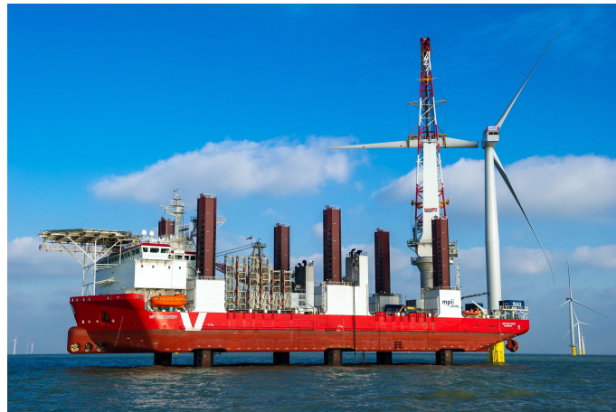
Figure 2.9: Self-propelled installation vessel (Offshore Wind Industry, 2013)
