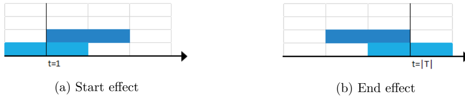
Figure 5.1: Illustration of the start effect and end effect when applying a time discrete optimization model
