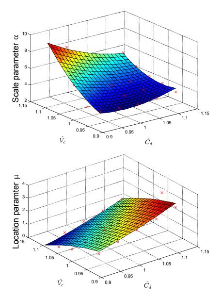
Figure 9: Response surfaces of Gumbel distribution parameters  $\alpha$  and  $\mu$  for the offset A = 5m.
