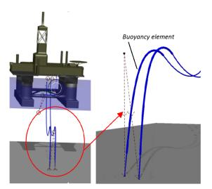
Figure 6: Model of the riser system.
