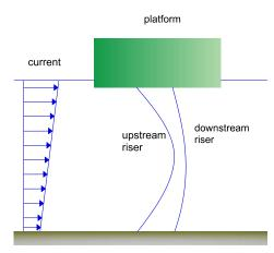
Figure 3: The static profile of risers when subjected to a current.
