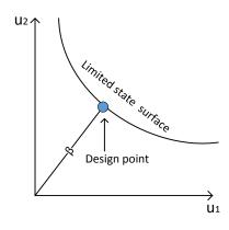
Figure 2: Failure surface and design point.
