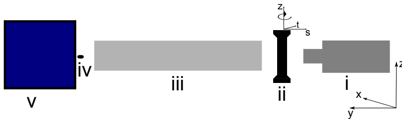
Figure 4.2: The experimental set up after the X-ray optics in Figure 4.1. i: X-ray optics, ii: sample, iii: flight tube, iv: beam stop, v: Pilatus 2M detector.
