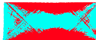
Reconstructed orientation distribution for the talc particles by SAXS tomography, using a model with only two (orthogonal) disk orientations. The directions of the talc flakes surface normal are given by the color wheel. It is noticed that the main features of the tomographically reconstructed distribution are qualitatively equal to the distribution measured by raster scanning.
