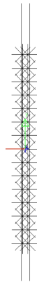
Figure 3.16: Line source with several 14^\circ point sources arranged in 0.2 \times 5 \text{ mm}^2 .
