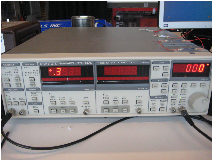
(a) Stanford SR830 DSP lock-in amplifier used to measure current and phase angle through the samples.
