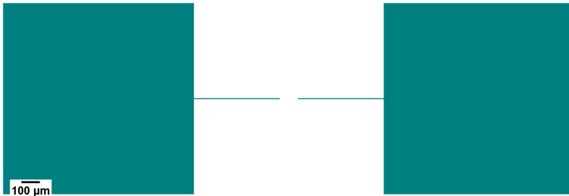
(a) Single electrode pair. The distance between the electrode tips is 100 \mu\text{m} .
