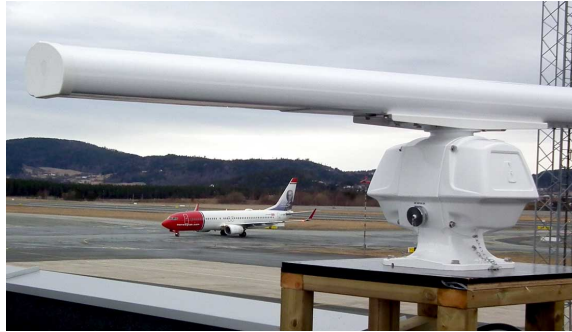
Figure 1.2: The birdstrike avoidance radar at Værnes Airport (deployed April 8th, 2014) used for measurements in this thesis. Here shown with an aircraft on the tarmac in the background.
