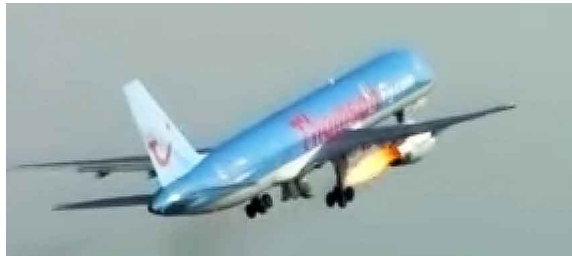
Figure 1.1: A Thomsonfly Boeing 757 right after suffering a double birdstrike (supposedly two herons) to the right engine causing engine failure during take-off from Manchester Airport in April 2007. The engine started to shoot large jets of flames, but was shut off. The aircraft turned and landed safely with one engine.[64][7]
