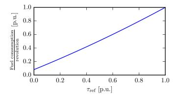
Fig. 2. Fuel consumption per revolution as a function of diesel engine's torque.
