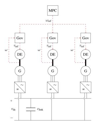
Fig. 1. Overview of the marine electric power plant without loads. The red dashed lines are signals, the thick lines are mechanical shafts, and the remaining lines represents electrical lines. Gov, DE, and G represents governor, diesel engine and generator. Loads are connected to the DC-link.
