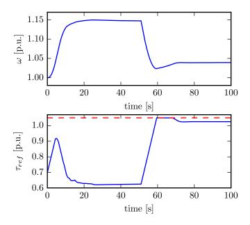
Fig. 6. Simulation of the power plant running with a load of 70%. One of the three connected generator sets is disconnected after 51 seconds. In the plot for  $\tau_{\rm ref}$ , the dashed red line shows the maximum diesel engine torque.
