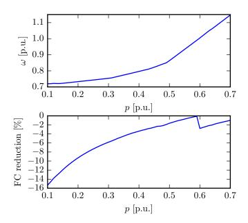
Fig. 7. The left plot shows the optimal steady state generator set speed as a function of the load. The right plot shows the reduction of fuel consumption with the proposed controller compared with running generator set at rated speed. Note that a new generator set must be started when the steady state speed is above the rated speed, this reduces the generators efficiency.
