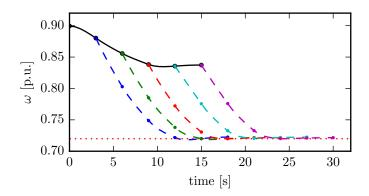
Fig. 4. Future trajectories for the generators' speed. The solid black line is the predicted trajectory of the nominal scenario. The dashed lines are the predicted fault scenarios, starting at  $t_f = 3$ , 6, 9, 12, 15 respectively. The dotted red line represents the under-speed limit which all trajectories should be above. An inter-sample violation of the constraints occurs as the constraints are only applied to the sample instants.
