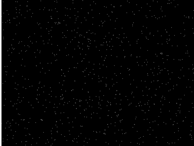
Figure 46: BW-image. White pixels represents identified edges from steep gradients in the pixel intensity still present after removal of hot pixels. 1252x1663 pixels
