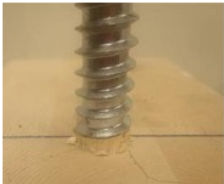
(a) Failure mode of specimen \alpha = 0^\circ
