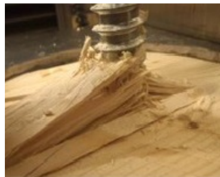
(b) Failure mode of specimen \alpha = 90^\circ
