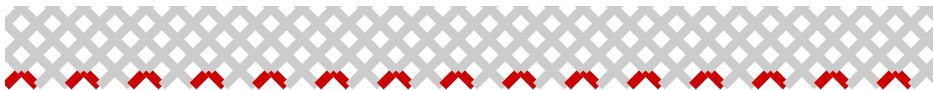
Figure 3.6: The initial and boundary conditions for the bottom rows of nodes. The non-wetting liquid is shown in red while the wetting liquid is shown in grey. The entire lattice is initially filled with wetting fluid while wetting and non-wetting fluid is injected simultaneously.
