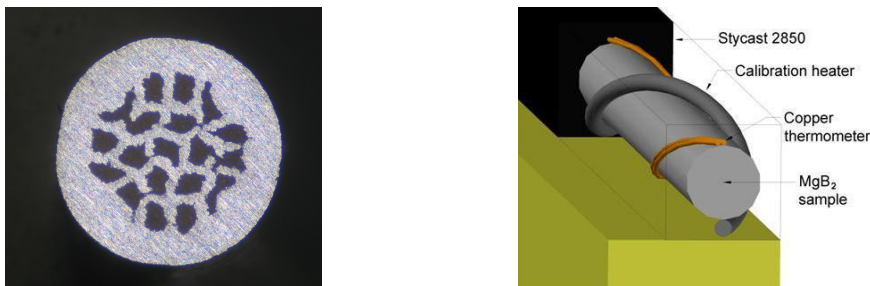
Figure 2. Cross-section of the sample wire (left) and the principle sample configuration (right) [16].
