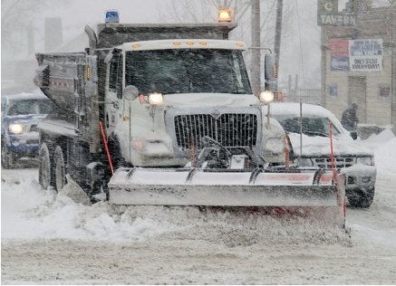
Figure 1.1: A snow plowing truck, plowing the outer of two lanes in the same direction. Photo: FEMA/ Michael Rieger, desaturated from original.
