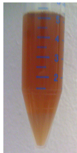
Figure 4.8: Sedimentation of particles in the buffer-esterase sample
