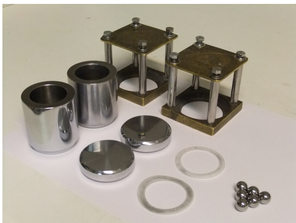
Figure C.3: The grinding bowls, the lids, the balls, the metal frames and the gaskets
