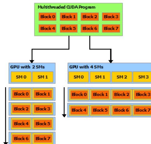
Figure 2.7: Distribution of blocks over the multiprocessors. Here, they are called streaming multiprocessors . The figure is taken from [2].
