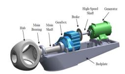
Figure 3. Drive train configuration of the NREL 750kW wind turbine [41]
