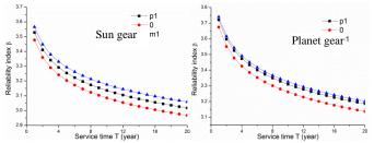
Figure 9. Reliability index  $\beta$  at 3 different contact points of the sun gear and the planet gear
