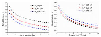
Figure 10. Reliability index  $\beta$  at the pitch contact point of the sun gear with respect to different values of  $a_0$  and  $a_c$
