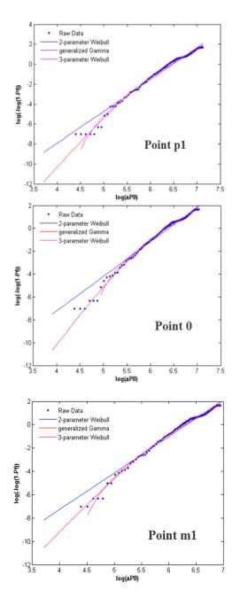
Figure 5. Long-term fitting results of  $\Delta p_{max}$  generated in the representative tooth of the planet gear
