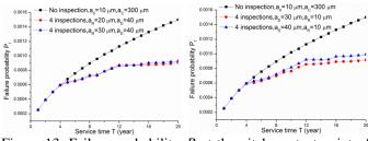
Figure 13. Failure probability  $P_f$  at the pitch contact point of the sun gear with respect to different  $a_R$  and  $a_D$  considering the effect of inspection
