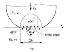
Figure 2. Orientation of the initial crack and contact loading
