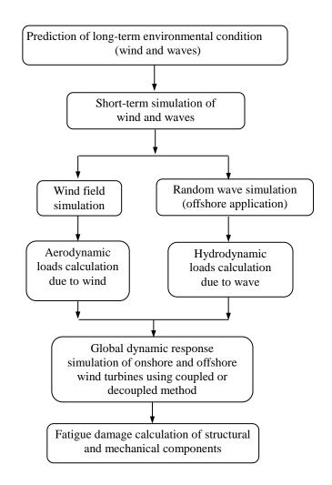
Figure 1: Schematic of the basic procedures in an integrated fatigue analysis based on time domain simulation
