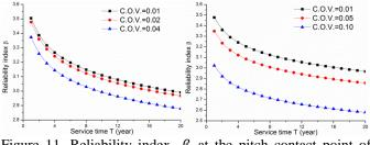
Figure 11. Reliability index  $\beta$  at the pitch contact point of the sun gear with respect to different C.O.V. of *lnC* and *lnA*
