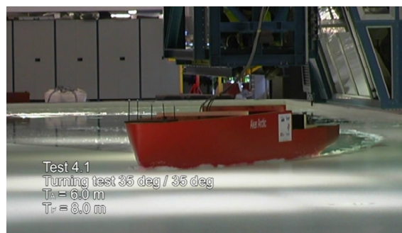
Figure 4. An example of the maneuvering tests in level ice (Source: Aker Arctic model test, Leiviskä, 2011).
