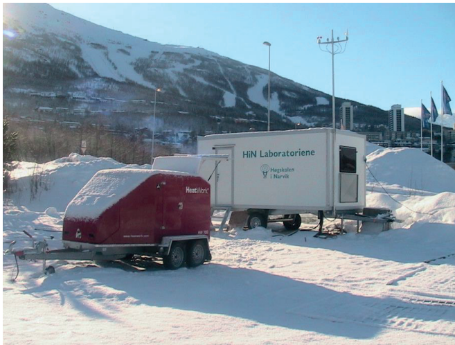
Figure 3. FiG-lab; Mobile measurement central (in the back) with a weather station attached, including a Heatwork defrosting machine (in the front). (Photo: Ø. Søråas)
