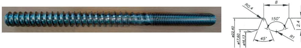
Figure 6: Purpose-made long threaded rods used in the investigation (left) and geometry of the wood thread (right). Measures given in mm.
