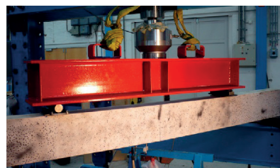
Fig. 4. Experimental set-up of beam splice test (dimensions given in mm).
