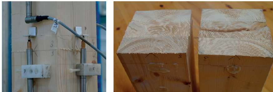
Fig. 9. Deformation of the crushing zone during testing (left), and deformation pattern at the end faces after testing (right).
