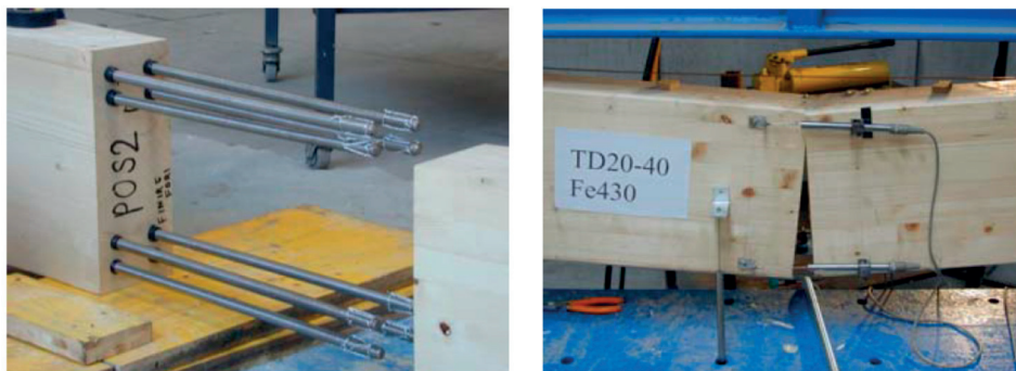
Figure 2.3 Splice joint with glued-in rods: rods glued into one member of the joint (left), deformation of the joint (right), [28]
