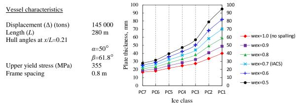
Figure 5. Effect of spalling parameter (*wex*) on the plate thickness.
