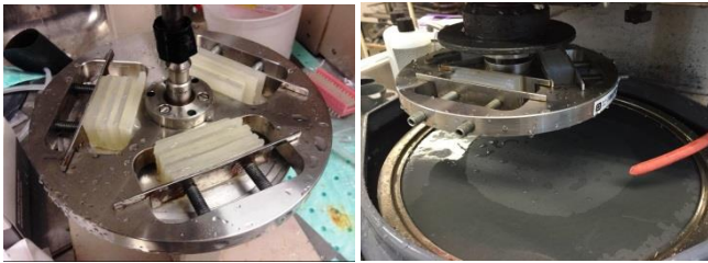
Figure 8. Surface preparation of the aligned and fixed specimens.
