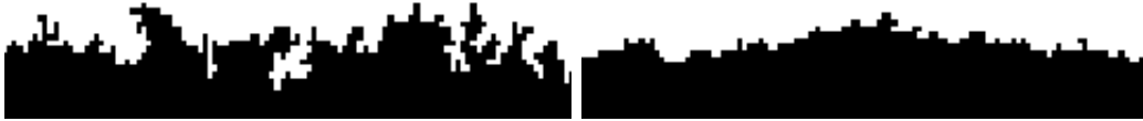
Figure 4.2: Snap-shots of fracture fronts from the simulations. The view is as seen from above in Figure 3.1. Black represents broken material and white is undamaged material. The left hand side shows small scale behaviour and the right hand side shows large scale behaviour. The fracture grows upwards.
