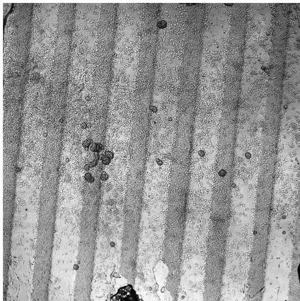
Figure 17: The lanes on patterned surfaces are easily distinguished in optically recorded images.
