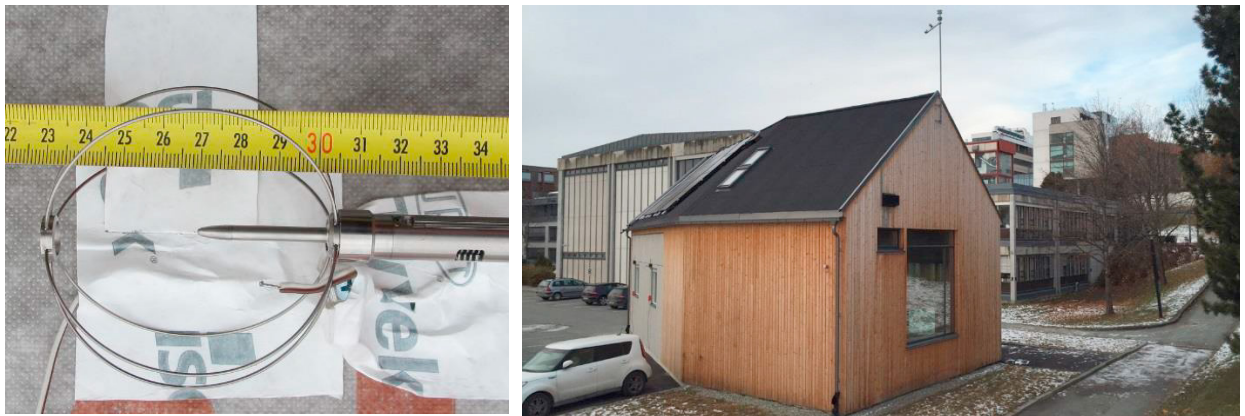
Fig. 1. Left: the omnidirectional air velocity measurement device. Right: the ZEB Test Cell Laboratory located at the NTNU campus in Trondheim. The weather station is positioned 10 m above ground level, 1.5 m above the ridge of the roof.
