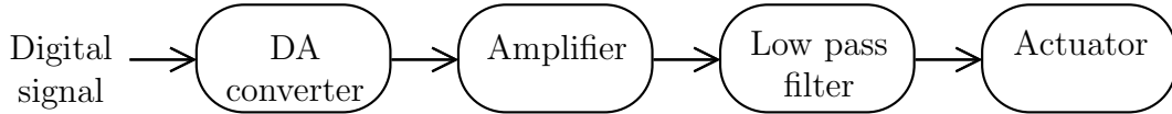
Figure 3.8: Schematic diagram of the signal flow in the electric circuit, from the computer to the piezoelectric actuators. The low-pass filter is only present for the scanning actuator.
