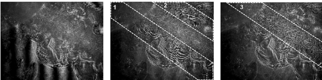
Figure 2.18: Topographic phase maps of a c-Si sawing channel for three scan positions. Left: Low frequent fringes are apparent in the lower left corner, corresponding to a flat surface. Middle: Fringes are present on the channel edges (1 and 2) only. Right: Fringes are present near the bottom of the channel. [Reprinted from Gastinger et al. [19]].
