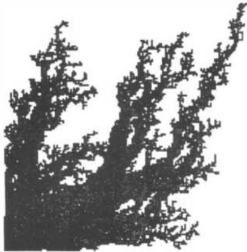
Figure 9: Numerical simulation of viscous fingering. Injection of a fluid of low viscosity (black) into a fluid of higher viscosity (white). Figure from Homsy [44]
